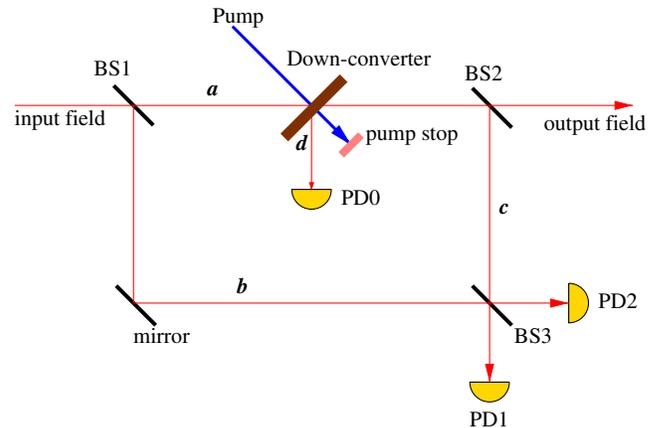
FIG. 1 (color online). Experimental setup. BS1 and BS2 are beam splitters of high transmittivity. A photon is added by a parametric down-converter between BS1 and BS2. A 50:50 beam splitter (BS3) superposes the reflected fields from BS1 and BS2. The output field is selected, conditioned on registering a photon at only one of the two photodetectors PD1 and PD2.  $a$ ,  $b$ ,  $c$  and  $d$  label the field modes.
