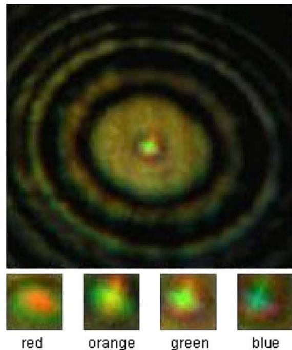
Fig. 5. Upper panel: Photograph of projections of the focal plane of the FZP in the region of the focal length for green wavelengths. Lower panel: Zoom-outs of the center of the focal planes for red, orange, green and blue wavelengths.
