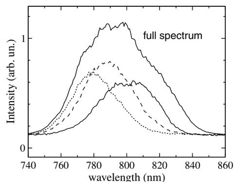
Fig. 2. Spectrum of the infrared laser beam after the FZP and selection with a 100  $\mu\text{m}$  pinhole at 108 cm (solid line), 115 cm (dashed line) and 122 cm (dotted line) from the FZP. The thin line shows the full spectrum (divided by 4).
