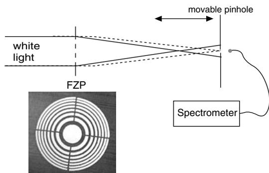
Fig. 1. Experimental set-up. The photo shows an optical image of a Fresnel zone plate consisting of 7 solid and 8 open rings with equal surface. The smallest structures are 100  $\mu\text{m}$ .
