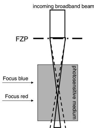
Fig. 6. Schematic representation of a device to simultaneously write and read information stored in wavelength channels of a broadband pulse using a FZP. The information is encoded in channels in the spectrum of the pulse as high or low spectral intensity. Different parts of the spectrum affect different spots in the medium where they are in focus.
