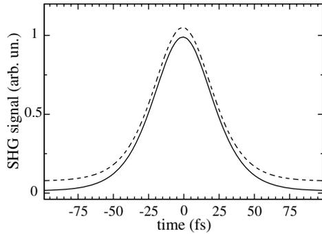
Fig. 3. Fits of a  $\text{sech}^2$ -function to the autocorrelation traces of the 800 nm pulses focused by a glass lens (solid line) and the FZP (dashed line). The traces are vertically offset for clarity. The pulse duration of  $\sim 65$  fs (full width at half maximum) is not considerably changed by the FZP.
