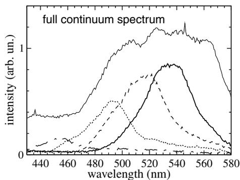
Fig. 4. Spectrum of the short-wavelength portion of the supercontinuum after the FZP and selection by a  $100 \mu\text{m}$  pinhole at a distance of 64 cm (solid line), 69 cm (dashed line), 74 cm (dotted line) and 82 cm (dash-dotted line) from the FZP. The thin line shows the full spectrum (amplitude divided by 2).
