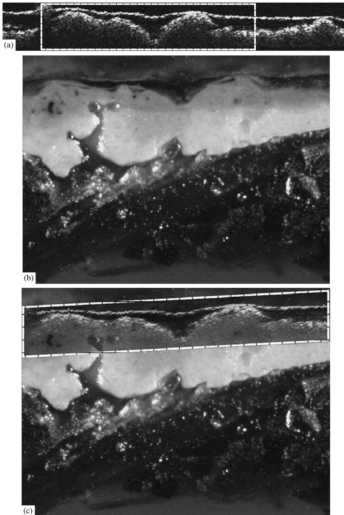
**Fig. 2.** (a) OCT image of a cross-section of the investigated area (dimensions: 2 mm length  $\times$  280  $\mu$ m depth). The varnish film surface (first from the top) and the paint layer surface are clearly visible. The dashed line selects the region that is common to the microscope image; (b) cross-section image acquired with a microscope after detaching the investigated volume; (c) superposition of the two images. OCT image has been tilted for proper alignment.
