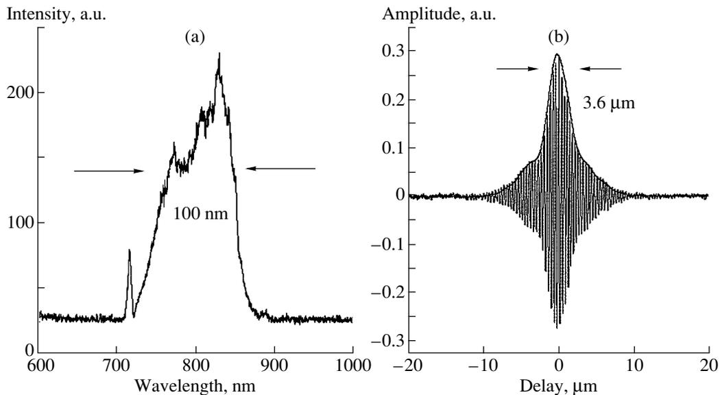
**Fig. 1.** (a) Spectrum of the Ti:Sa laser; (b) corresponding autocorrelation signal.
