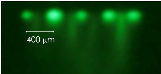
FIG. 2. (Color online) Picture of the harmonic generation region in the 5-hole gas jet configuration; the plasma light generated by intense laser ionization is evident in correspondence with the gas jets, separated by about  $400 \mu\text{m}$ .
