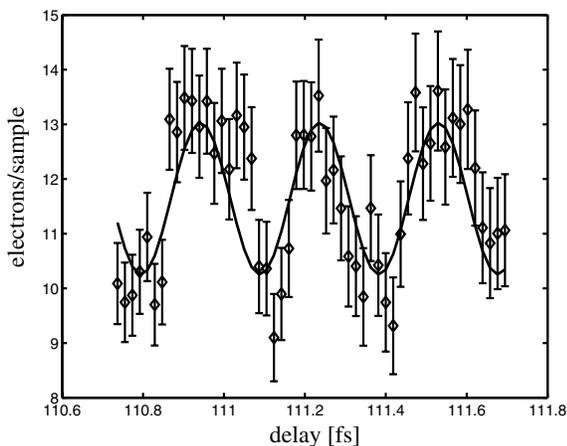
FIG. 3. Detail of the fringe pattern around the 110 fs delay. The fringe spacing corresponds to the 0.29 fs-period of the atomic transition. Experimental points result from summing over ten laser pulses and smoothing on a small fraction ( $\approx 10\%$ ) of the fringe period. The data bars measure the statistical errors.
