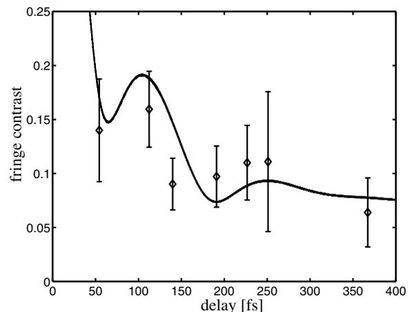
FIG. 4. Fringe contrast vs pulse delay. The solid curve superimposed to the data points is a theoretical curve, as explained in the text, where atomic parameters are obtained by the synchrotron radiation measurements of Ref. [12]. A single free parameter, corresponding to the ratio between the electron emission probabilities of the  $8s'$  and  $6d'$  states in the laser polarization direction, has been used in the fit.
