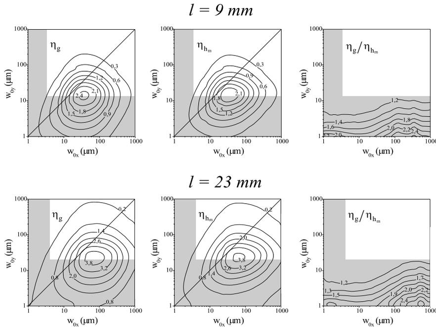
**FIGURE 3** Evaluation of the second harmonic generation efficiencies in the case of elliptical focusing. *Left-hand column:* efficiency  $\eta_g$  evaluated using our simplified formulas; *center column:* efficiency  $\eta_{\text{hm}}$  evaluated following B-K theory; *right-hand column:* ratio  $\eta_g/\eta_{\text{hm}}$ . In the grey regions agreement between the values of  $\eta_g$  and  $\eta_{\text{hm}}$  is not expected (see text)
