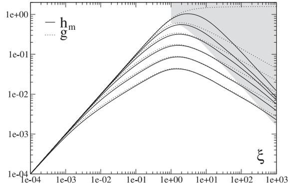
**FIGURE 1** Comparison between the Boyd–Kleinman function  $h_m(\xi)$  (continuous lines) and the function  $g(\xi)$  given by our simplified approach (dashed lines), for several values of the walk-off parameter  $B$ . Top to bottom curves:  $B = 0, 1, 2, 4, 8, 16$ . In the grey region the approximations leading to the evaluation of  $g$  are not valid
