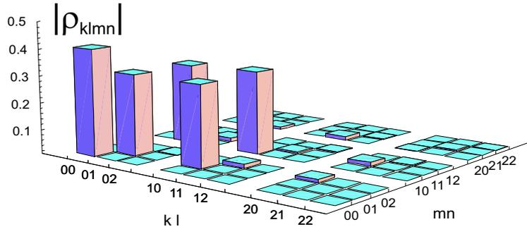
Figure 3. Reconstructed density matrix elements  $\rho_{klmn} = \langle k_1 l_2 | \hat{\rho} | m_1 n_2 \rangle$  corresponding to the state of Eq. (2) with  $\phi_i = 0$ .
