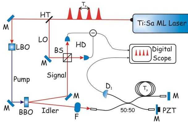
Figure 1. Schematic representation of the experimental setup. 50:50 is a 3 dB fiber coupler, HT a high-transmission beam splitter, and M are mirrors.
