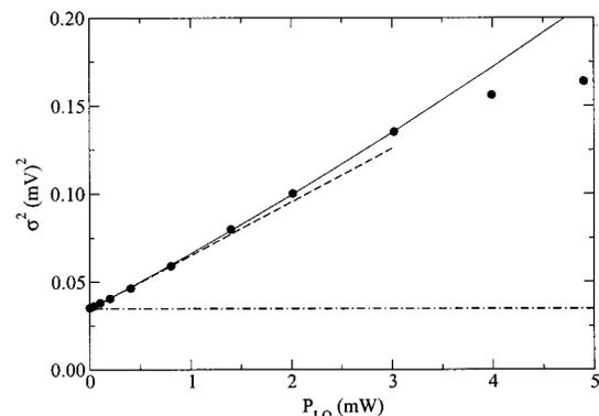
Fig. 3. Filled circles, integral of the power spectrum; solid curve, quadratic fit; dashed curve, shot-noise contribution; dashed-dotted curve, electronic noise.
