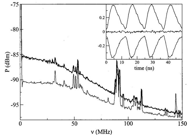
Fig. 2. Thicker curve, spectral power of the detected signal when one photodiode is illuminated by thermal light, giving a photocurrent of 1.16 mA. The resolution bandwidth is 300 kHz. Thinner curve, electronic noise. The narrow peaks are due to pickup from environmental noise. Inset, time-domain output signal with the laser impinging on only one photodiode (the upper and the lower traces correspond to the signals from the two detectors) and on both photodiodes (middle trace).
