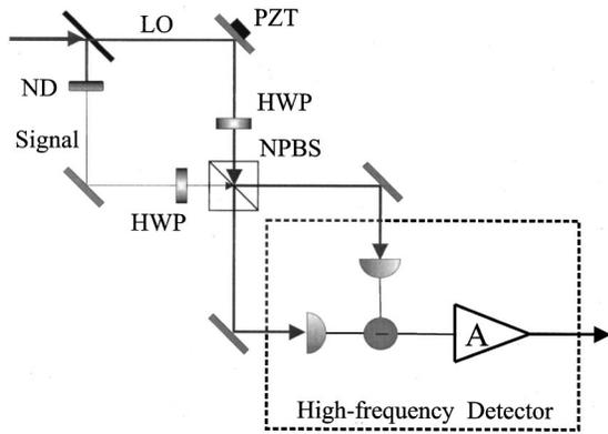
Fig. 1. Experimental setup: HWPs, half-wave plates; NPBS, nonpolarizing beam splitter; A, amplifier; PZT, piezoelectric translation stage; ND, neutral-density filter.
