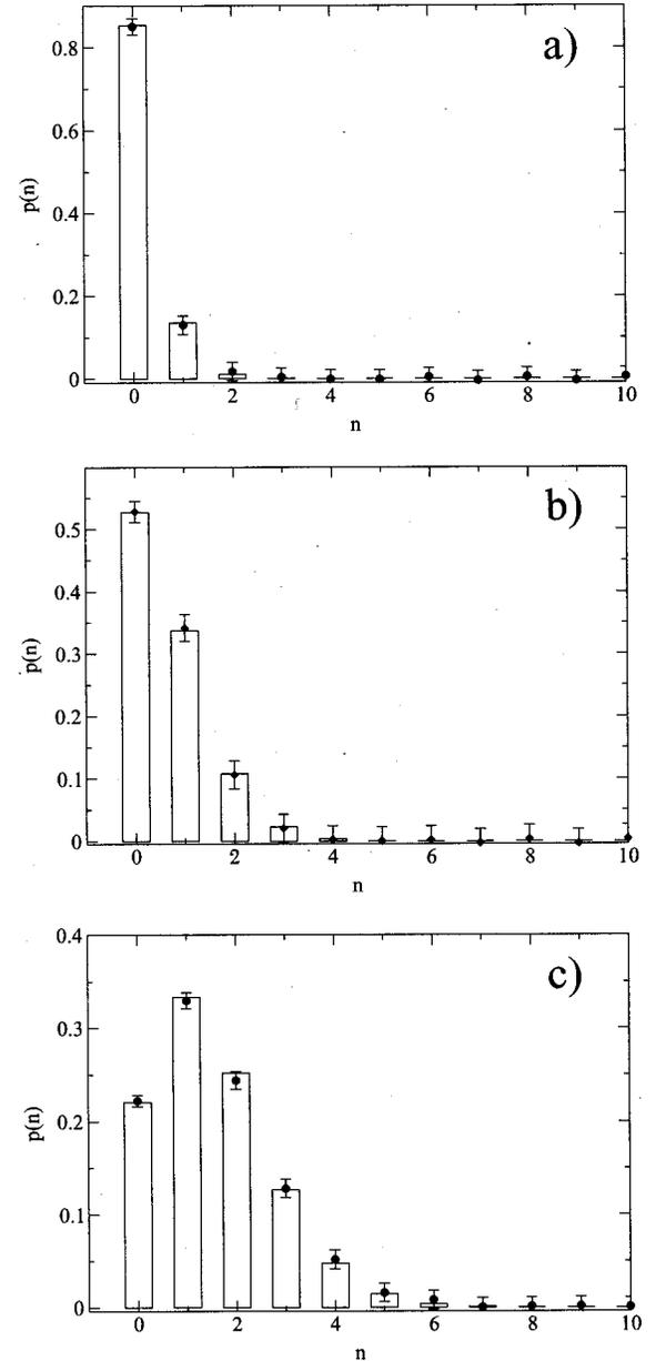
Fig. 7. Reconstruction of the photon statistics of three coherent states. The filled circles with error bars are the reconstructed values. Rectangles, best-fit Poissonian distribution values with (a)  $\langle n \rangle = 0.16$  photons/pulse, (b)  $\langle n \rangle = 0.64$  photons/pulse, and (c)  $\langle n \rangle = 1.5$  photons/pulse.
