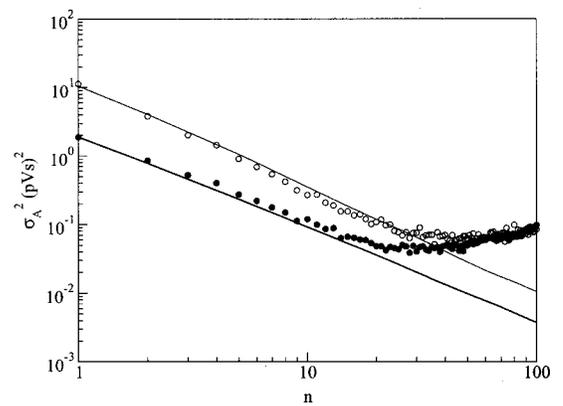
Fig. 5. Allan variance of the pulse energy. Open circles, laser power of 3 mW; filled circles, electronic noise; solid curves, Allan variances calculated from the spectrum according to Eq. (4). The abscissa is in units of pulse separation  $T$ .
