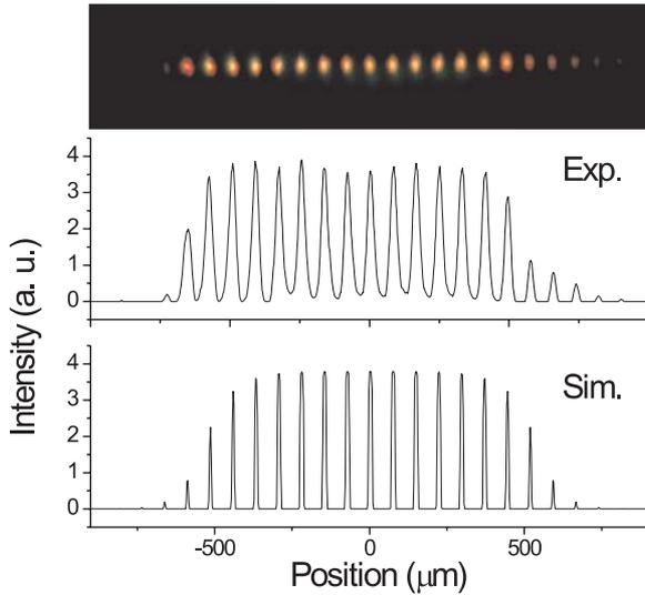
**FIGURE 3** Experimental CCD image of the supercontinuum array source region. Also reported are the profiles obtained by a horizontal cut across the image and the simulated supercontinuum intensity distribution from (4), (5), and (6). An array of about 15 white-light sources of almost constant intensity is produced in this case
