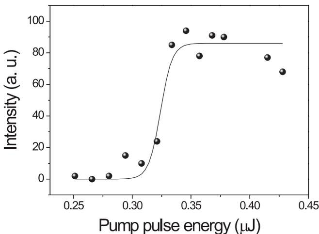
**FIGURE 2** Behavior of the supercontinuum intensity variation as a function of the incoming laser power for a wavelength of about  $550 \text{ nm}$ . Filled circles are experimental data while the solid line is a fit with the hyperbolic tangent function (6) used to model this behavior
