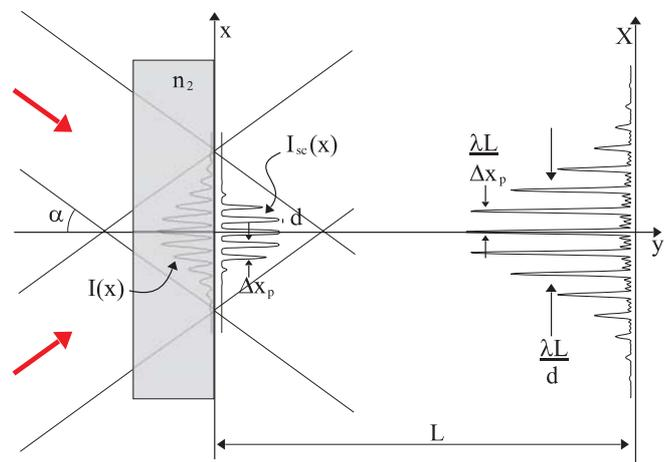
**FIGURE 1** Sketch of the experimental setup illustrating the geometry of the interaction. Two laser pulses intersect at an angle  $\alpha$  and form an interference pattern on the  $x$  plane inside the material. The maxima of this interference pattern become the sources for supercontinuum radiation which propagates to a screen placed at a distance  $L$
