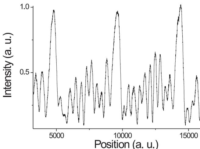
**FIGURE 5** Same as Fig. 4 but with a higher pulse energy. More white-light sources (at least 15) are present with a more pronounced phase distribution which gives rise to distortions in the interference profile
