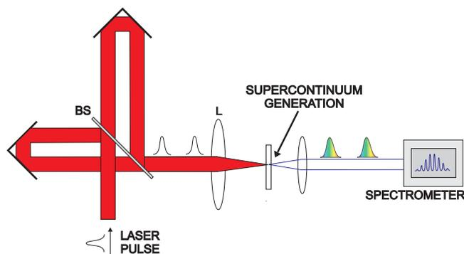
**FIGURE 1** Experimental setup for the test of the phase-lock between collinear white-light continuum pulses. The IR pulses from the laser were split and recombined by a 50% beamsplitter (BS) and focused with a variable relative delay  $\tau$  by the lens L in a glass plate. Frequency-domain interference fringes were detected by a spectrometer
