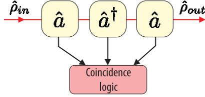
Fig. 2. – Combination of three quantum operations: single-photon addition between two single-photon subtraction stages. By the right combination of “clicks” from the detectors it is possible to select the desired  $\hat{a}\hat{a}^\dagger$  or  $\hat{a}^\dagger\hat{a}$  sequences.
