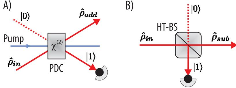
Fig. 1. – Schemes for the conditional implementation of single-photon addition (A) and single-photon subtraction (B). The detection of a single-photon heralds the preparation of the photon-added or photon-subtracted state.
