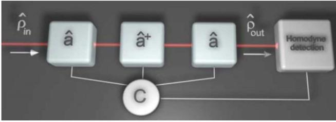
**Figure 1.** Block diagram of the experiment for the test of non-commutativity between creation and annihilation operators.
