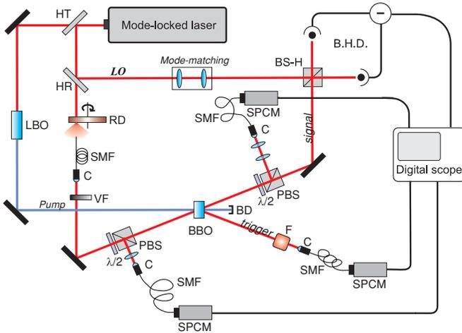
**Figure 2.** Scheme of the complete experimental setup. Most symbols are defined in the text. BBO indicates the beta barium borate SPDC crystal. The beam splitters for photon subtraction are composed of a half-wave plate ( $\lambda/2$ ) and a polarizing beam splitter (PBS) for accurate adjustments of their transmissivity. C stands for collimating (collecting) optics for single-mode fibres (SMF). SPCM: on/off detector, HT (HR): high-transmissivity (reflectivity) mirror, BD: beam dump.
