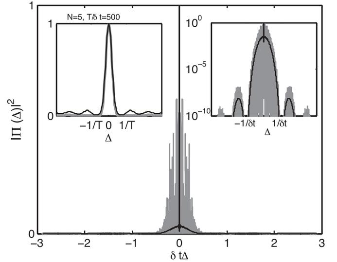
FIG. 3. Plot of the squared magnitude of the product of the Fourier transform of  $N$  couples [Eq. (7)] at random delays, and of the mean value [Eq. (8)]. Here  $N = 5$  and  $T = 500\delta t$ . In the inset on the left, the mean value is barely discernible from the random extraction.
