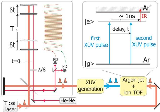
Fig. 1. (Color online) Scheme of the experimental setup. Left inset: Michelson interferometer and scheme of the two-time-window measurement. Right inset: relevant Ar levels and pulse sequences.
