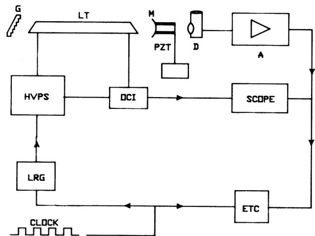
FIG. 1. Experimental setup. LT, laser tube; G, grating; M, mirror; PZT, piezoelectric translator; HVPS, high voltage power supply; OCI, optically coupled isolator; LRG, linear ramp generator; ETC, electronic time counter; D, Hg-Cd-Te detector; A, low-noise amplifier.
