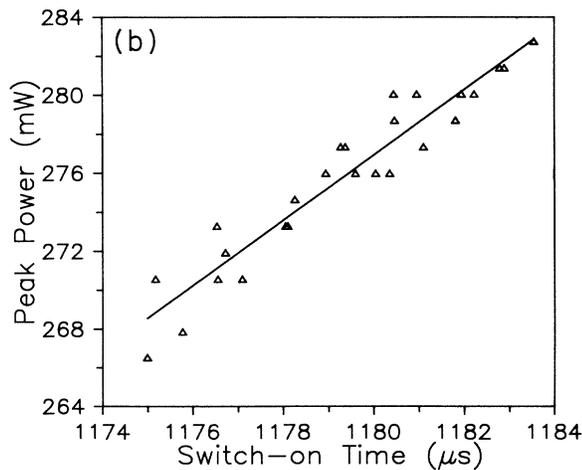
FIG. 2. (a) Switching events obtained for  $\theta_1 = 3.80$  A/s. (b)  $I_m$  vs the switch-on time  $T$  for  $\theta_1 = 3.80$  A/s ( $I_{th} = 5$  mW). The best fit line slope is 1673 W/s.
