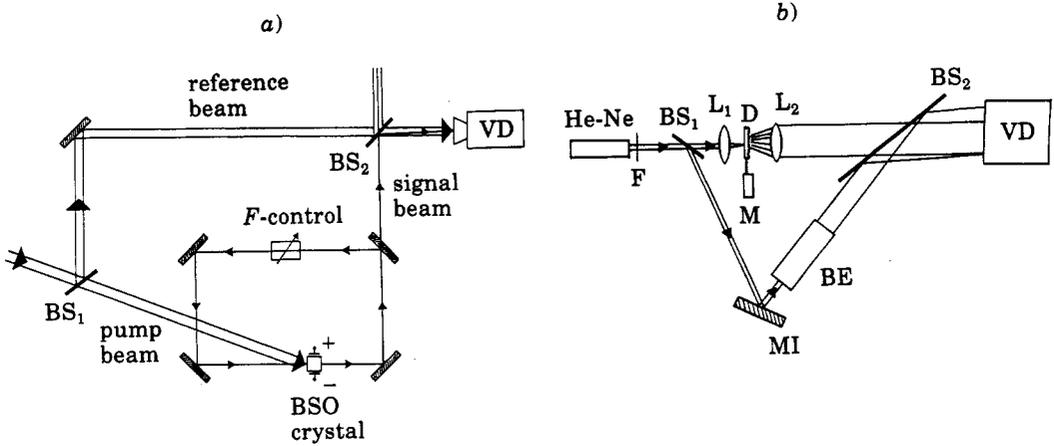
Fig. 1. - Experimental set-up for *a*) the nonlinear experiment and *b*) the linear experiment; VD is a CCD videocamera.
