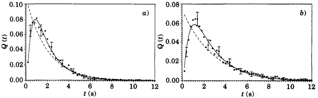
Fig. 4. - Probability of having 0 successive events within a time  $t$  counted from an initial time  $t_0$  corresponding to an event. The data refers to a) the nonlinear case and b) the linear case; the strong deviations from the dashed lines (Poissonian fits) are due to the refractory time in the time series. Solid lines correspond to the best fit of eq. (5) with the data.
