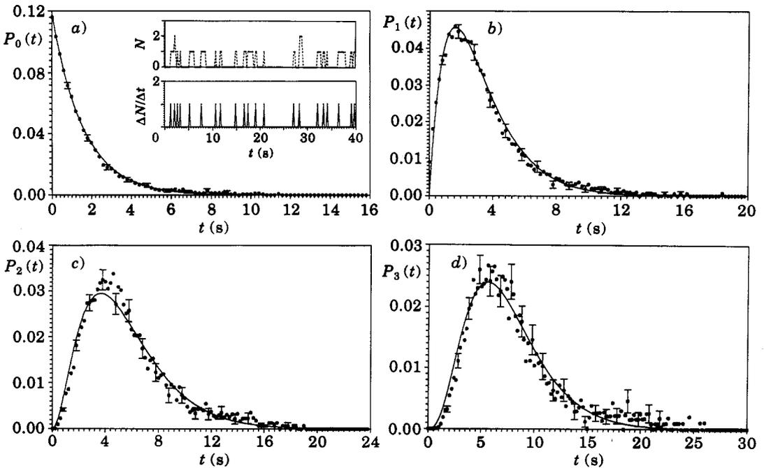
Fig. 3. - Probabilities of having a) 0, b) 1, c) 2, d) 3 successive events within a time  $t$  starting from a random initial time  $t_0$ ; an event is the entrance of a defect into a correlation domain and the data refer to the nonlinear experiment. For convenience, error bars have been reported every five points. Inset: time sequences of (above) permanence of a defect in a correlation domain and of (below) entrance of a defect in the same domain.
