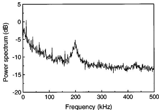
FIG. 6. Power spectrum of the local laser intensity.
