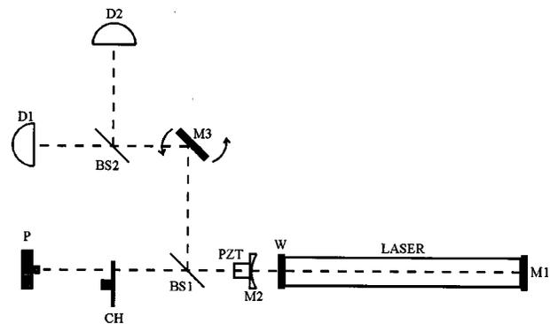
FIG. 1. Experimental setup. *M1*: total reflective mirror; *W*: ZnSe antireflection window; *M2*: Ge outcoupler mirror mounted on a piezo translator (PZT); BS1 and BS2: ZnSe beam splitters; CH: mechanical chopper; *P*: pyroelectric array detector; *D1* and *D2*: single element Hg<sub>x</sub>Cd<sub>1-x</sub>Te detectors.
