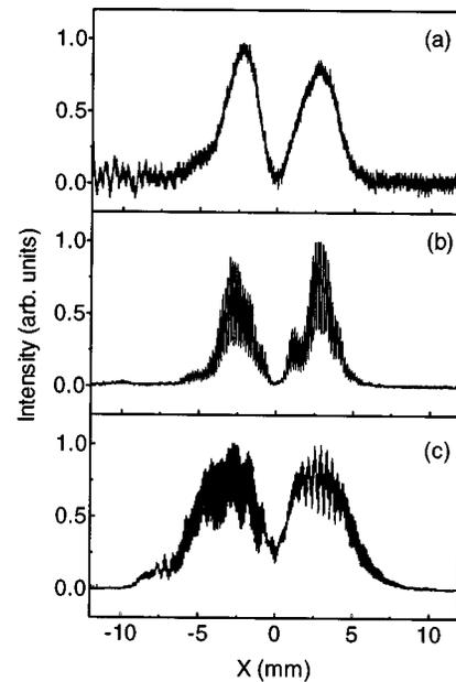
FIG. 3. Experimental transverse profiles of the pattern of Fig. 2(a) detected by (a) the linear pyroelectric array, (b) the  $\text{Hg}_x\text{Cd}_{1-x}\text{Te}$  detector with a  $200\ \mu\text{m}$  pinhole, and (c) the  $\text{Hg}_x\text{Cd}_{1-x}\text{Te}$  detector without pinhole.
