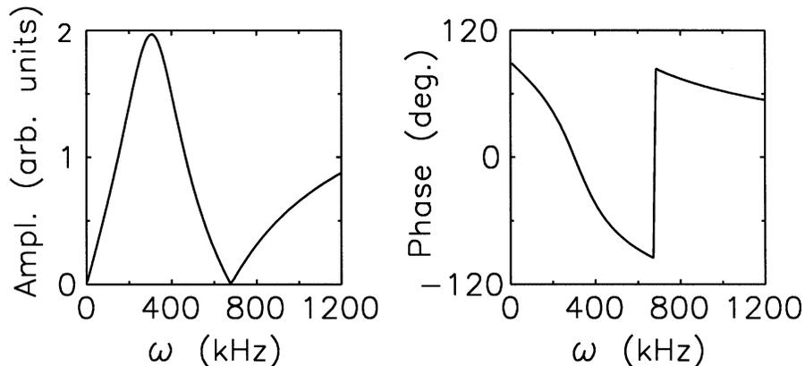
Fig. 1. Amplitude and phase response curves of the washout filter as a function of  $\omega$ .
