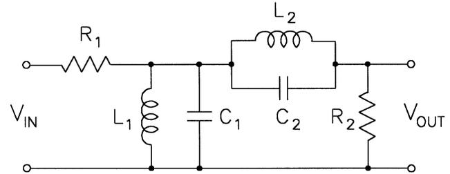
Fig. 6. Electronic scheme of the washout filter:  $R_1 = 1$  k $\Omega$ ,  $L_1 = 6.5$  mH,  $C_1 = 0.1$  nF,  $R_2 = 6.7$  k $\Omega$ ,  $L_2 = 12.4$  mH and  $C_2 = 0.2$  nF.
