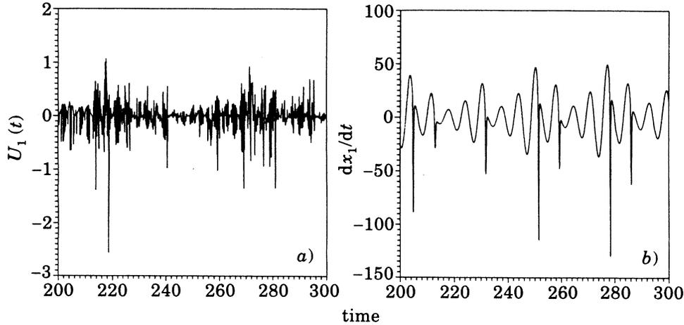
Fig. 5. (a) Temporal evolution of the first component of the additive controlling term  $U_1$  during the control of period-8 of Ro4 and (b) temporal evolution of the uncontrolled  $dx_1/dt$ . The adaptive correction term is between two and three orders of magnitude smaller than the natural evolution of the dynamics. Same stipulation for controlling task as mentioned in the caption of Fig. 4.
