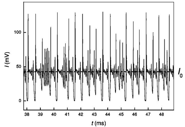
FIG. 3. Portion of time series for chaotic window  $C^5$ . For calculating RMRT, the signal is sampled at  $I_0 = 44$  mV.
