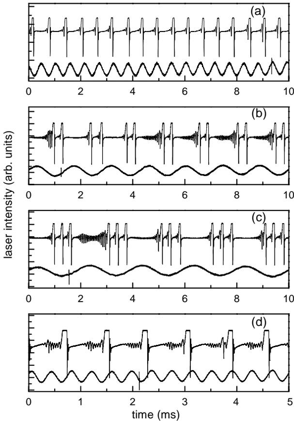
Fig. 3. Experimental time series for different phase synchronizations induced by a frequency modulated control parameter. For comparison, time plots of the modulation control parameter are reported in each case. The modulation frequencies are respectively (a) 1:1 at 1.6 kHz; (b) 1:2 at 0.7 kHz; (c) 1:3 at 0.5 kHz; (d) 2:1 at 2.6 kHz.
