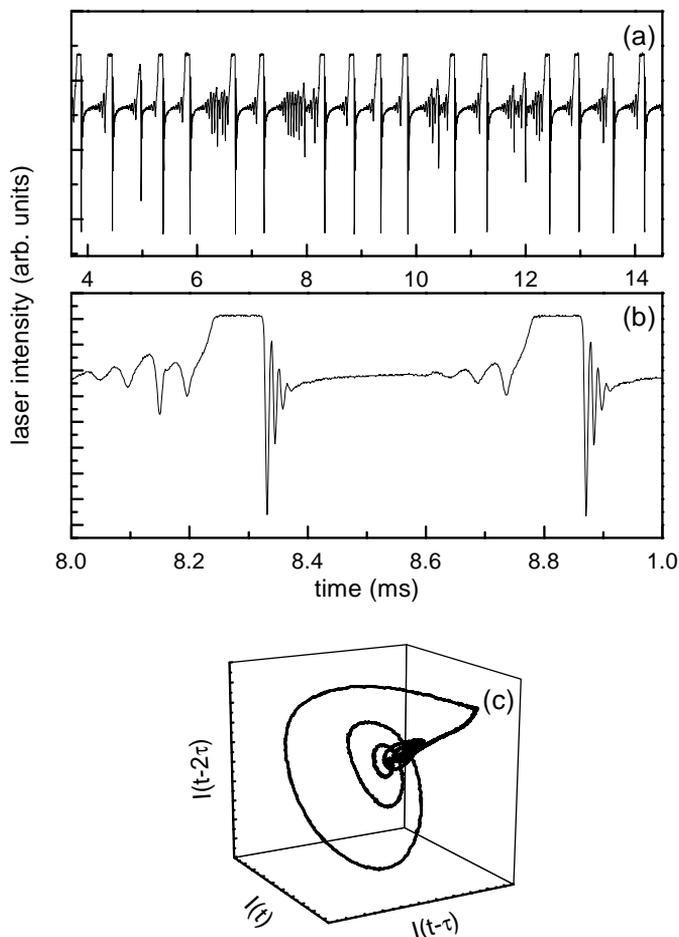
Fig. 2. (a) Experimental time series of the laser intensity for a CO<sub>2</sub> laser with feedback, in the regime of homoclinic chaos. (b) Time expansion of a single orbit. (c) Trajectory built by an embedding technique with appropriate delays.
