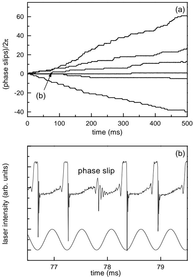
Fig. 5. (a) Phase slips at different frequencies for the 20 mV amplitude (horizontal line B in Fig. 4(a)). The dynamical system monotonically lags or leads in phase depending on whether the modulation frequency is above or below the perfect synchronization (no slips) value of 1.6 kHz. (b) Expanded view of the time in a phase slip. The phase slip is like a defect in a periodic one-dimensional pattern; in fact in this case it is a missed return to the surface of section.
