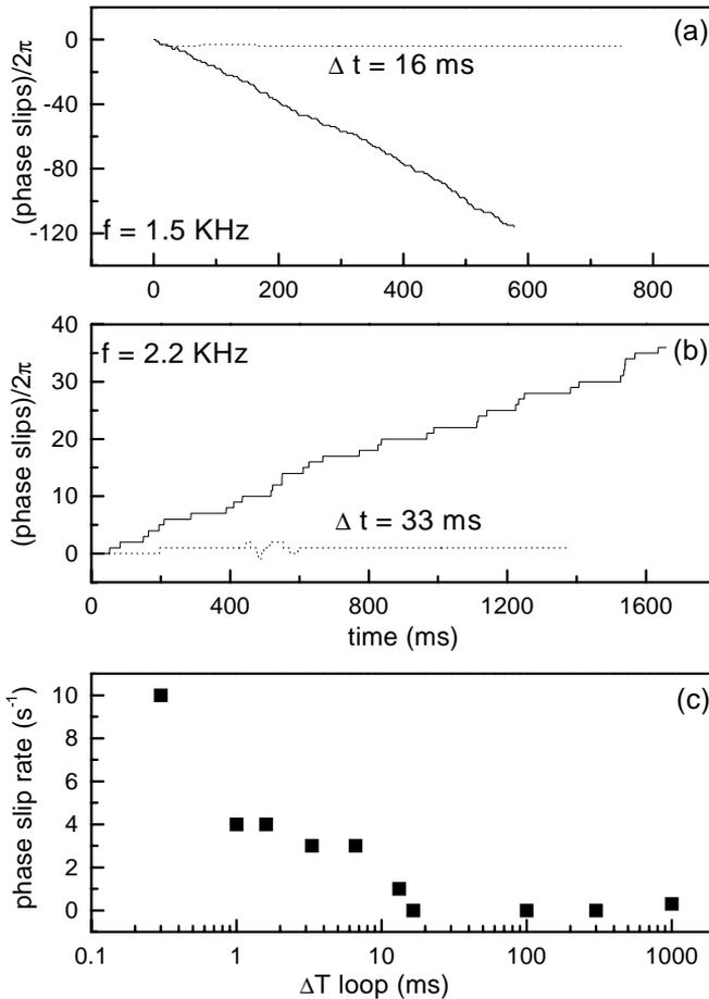
Fig. 6. Long time correction of the phase slip in two cases where the uncontrolled frequency setting of the modulation is below (a) or above (b) the frequency corresponding to the perfect synchronization, solid and dotted lines represent the uncontrolled and controlled case, respectively. (c) Dependence of the residual phase slip upon the sampling time in case (b).
