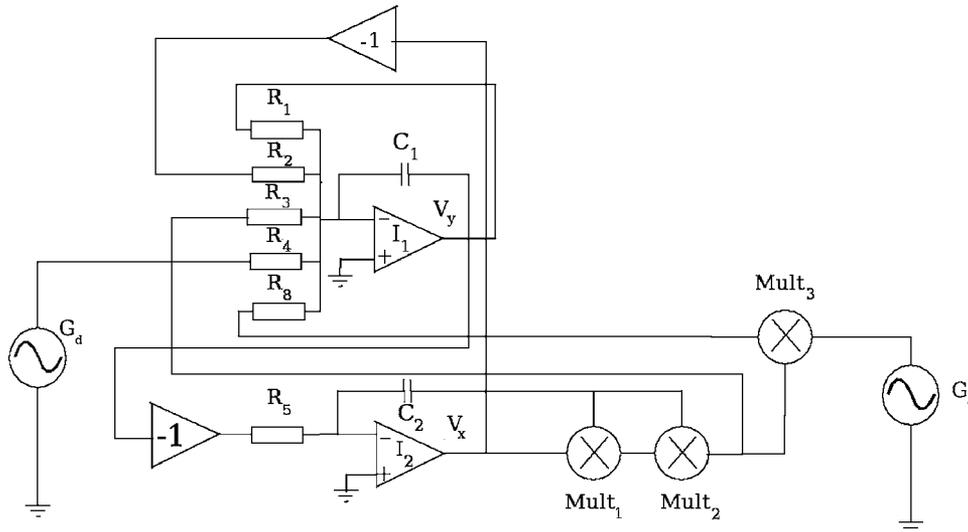
FIG. 6. Sketch of the electronic circuit. *I*: integrators; *R*: resistors; *C*: capacitors, Mult: multipliers;  $G_d$ : sinusoidal wave generator;  $G_c$ : arbitrary wave form generator. Under a suitable time normalization, the dynamics of the circuit is given by  $\ddot{x}+0.1471\dot{x}-x+(1+\epsilon\cos(r1.257t+\phi))x^3=0.263\cos(1.257t)$ , where  $x \propto V_x$  and  $\dot{x} \propto V_y$ . The  $\epsilon, \phi, r$  values can be fixed with the arbitrary wave form generator.
