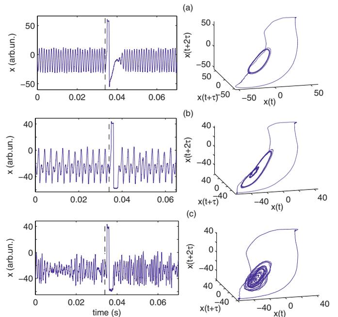
**Fig. 2.** (Color online) Left panels: Experimental time series for the laser intensity for different parameters. The external perturbation in the form of a sharp pulse (duration 1 ms) has been added to the pumping current at time marked by the vertical dashed line. Right panels: Reconstructed phase space for the laser intensity by embedding method.
