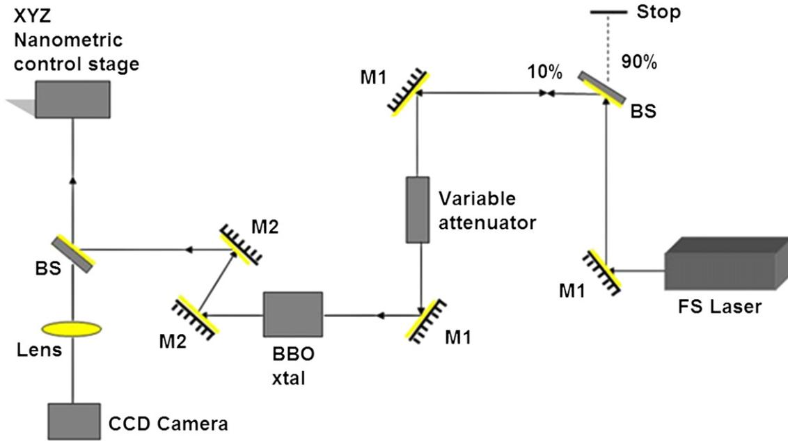
Fig. 1. The experimental setup of sub surface irradiation technique, M<sub>1</sub> 50 mm diameter IR mirrors, and M<sub>2</sub> 50 mm diameter UV mirrors.
