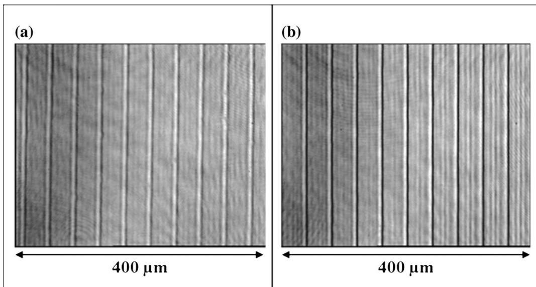
Fig. 2. Top views of the UV written phase gratings in PMM with a scan speed of 1.25 mm/s: (a) pulse energy of 0.102 μJ and 5 overscans, and (b) pulse energy of 0.105 μJ and 32 overscans.
