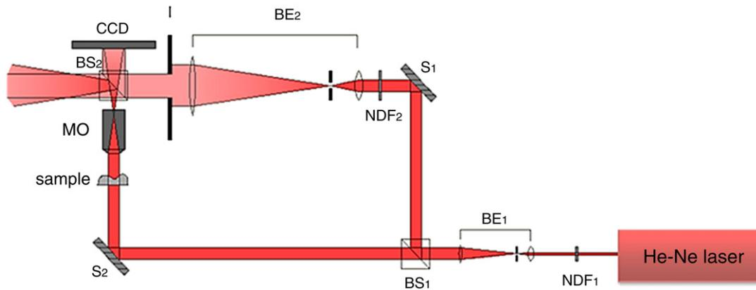
**Fig. 3.** Mach-Zehnder interferometric system in microscopic configuration. BS<sub>1</sub> and BS<sub>2</sub> are beam splitters. NDF<sub>1</sub> and NDF<sub>2</sub> are neutral density filters; BE<sub>1</sub> a spatial filter and beam expander for the incident laser light; BE<sub>2</sub> a spatial filter and beam expander to generate a plane wave front reference beam, and MO a microscope objective 10×.
