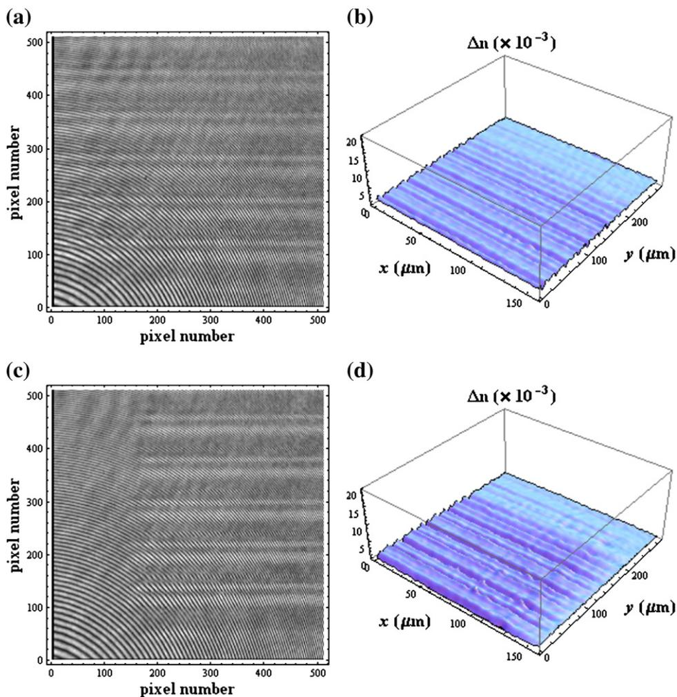
**Fig. 4.** 3D visualization of the spatial distribution of the index of refraction calculated from the interference patterns: (a) and (c) digitized interferograms of UV written phase gratings in PMMA with a scan speed of 1.25 mm/s and (b) and (d) corresponding refractive index maps.
