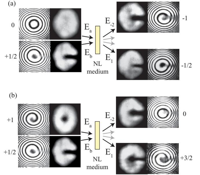
FIG. 4. (Color online) Vortex interaction for fractional input charges. Left: input beams  $E_a$  and  $E_b$  (phase, intensity); right: output beams  $E_1$  and  $E_{-2}$  (intensity, phase) with new topological charges; (a)  $l_a = 0$ ,  $l_b = +1/2$  and  $l_{-2} = +1$ ,  $l_{+1} = -1/2$ ; (b)  $l_a = +1$ ,  $l_b = +1/2$  and  $l_{-2} = 0$ ,  $l_{+1} = +3/2$ .
