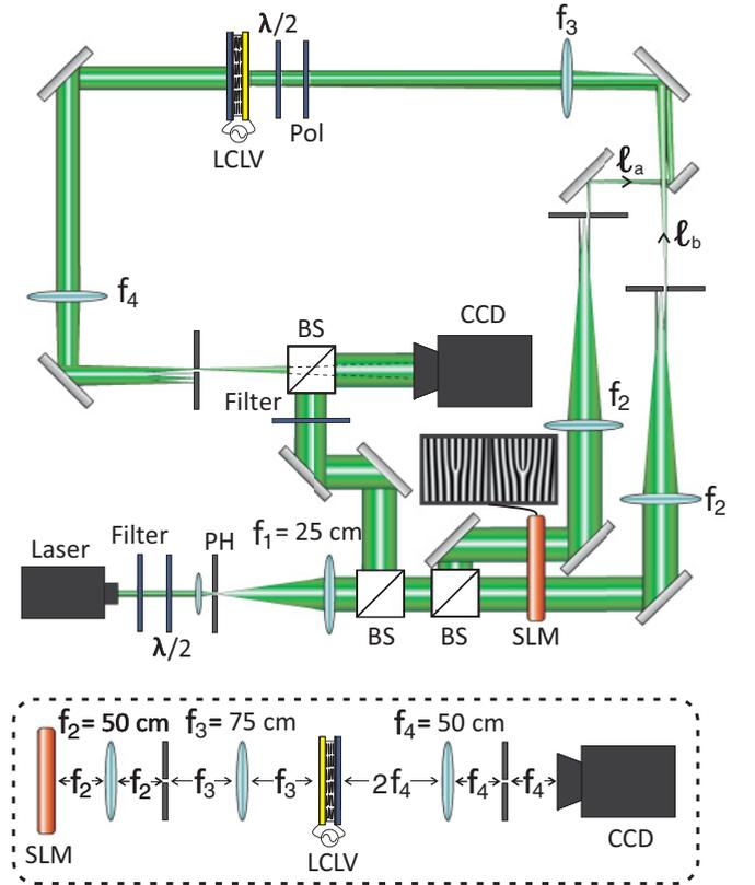
FIG. 2. (Color online) Experimental setup: the input laser is divided into two beams, each passing through the spatial light modulator (SLM) where the input vortex beams  $E_a$  and  $E_b$  are synthesized through holographic masks; the two beams are then sent to interact in the LCLV; PH, pinhole; BS, beam splitter. The bottom inset shows the self-imaging system before and after the LCLV.
