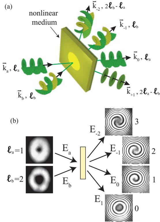
FIG. 1. (Color online) (a) Principle scheme of the vortex interaction for  $l_a = 1$  and  $l_b = 2$ , and (b) experimental snapshots showing the intensity of the input beams and the phase profiles of the corresponding output beams.
