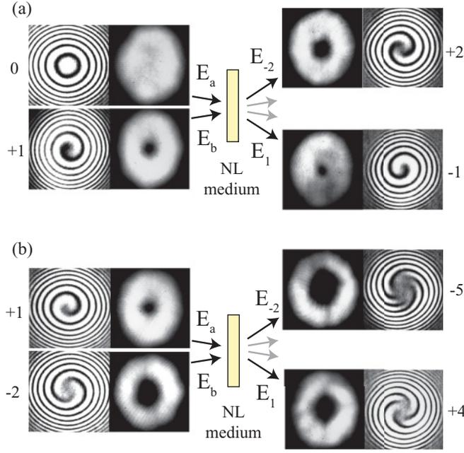
FIG. 3. (Color online) Vortex interaction for integer input charges. Left: input beams  $E_a$  and  $E_b$  (phase, intensity); right: output beams  $E_1$  and  $E_{-2}$  (intensity, phase) with new topological charges; (a)  $l_a = 0$ ,  $l_b = +1$  and  $l_{-2} = -1$ ,  $l_{+1} = +2$ ; (b)  $l_a = +1$ ,  $l_b = -2$  and  $l_{-2} = -5$ ,  $l_{+1} = +4$ .
