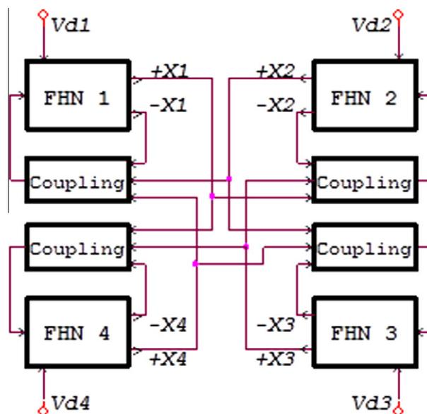
Fig. 1. Scheme for the network of four FHN. The coupling is bidirectional and the topological structure represents a ring.
