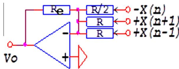
Fig. 3. Scheme for the electronic coupling.  $R_e$  e  $R$  denote resistors that control the coupling strength between the nodes.
