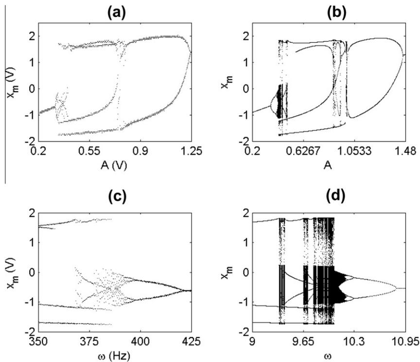
**Fig. 4.** Bifurcation diagrams for a single driven FHN as different control parameters vary: (a) and (b) amplitude  $A$  of the driving signal, (c) and (d) frequency of the driving signal. Diagrams in (a) and (c) are obtained experimentally and (b) and (d) numerically.
