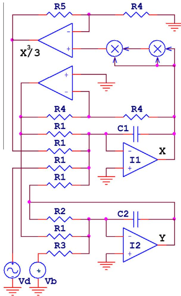
Fig. 2. Scheme of the electronic circuit implementing each driven FHN, with letters denoting  $I_k$  integrators,  $R_k$  resistors,  $C_k$  capacitors,  $X$  multipliers,  $V_d$  sinusoidal forcing signal and  $V_b$  fixed bias voltage.
