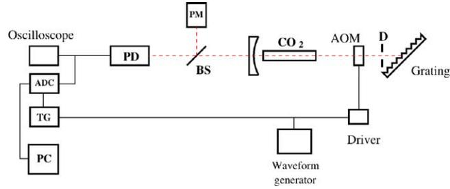
Fig. 1. Experimental apparatus used to perform our measurements. AOM: acousto-optic modulator; BS: beam splitter; PM: power meter; PD: photodetector; TG: trigger generator; ADC: analog to digital converter; PC: personal computer.
