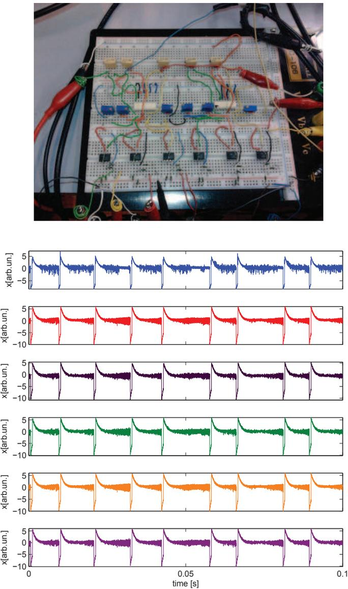
Fig. 7. Synchronization of six asymmetrically coupled chaotic LEDs.
