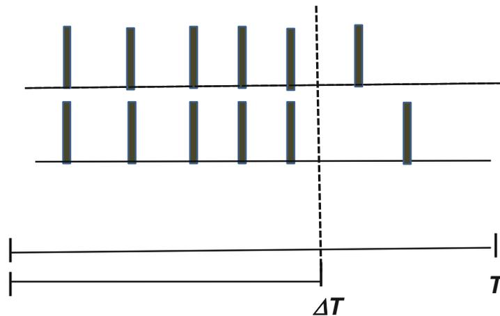
**Fig. 8.5** Two spike trains of duration  $T$ , synchronized up to  $\Delta T$ . The number of different realizations is  $2^{(T-\Delta T)}$
